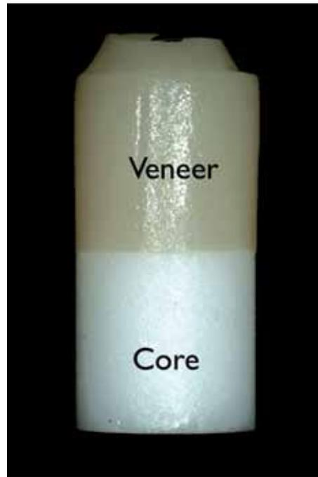
1 Example of specimen: zirconia ceramic group (pressed).
